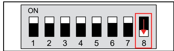
Figure 6-74 DIP SW1 #8 OFF for DS1 Testing
